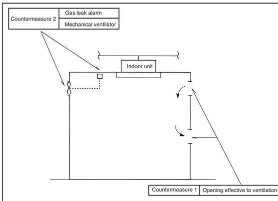
Pay a special attention to the place, such as a basement, etc. where refrigerant can stay, since refrigerant is heavier than air.
