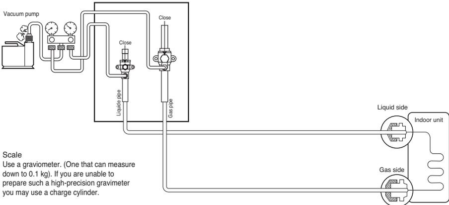
**Note : Always add an appropriate amount of refrigerant. (For the refrigerant additional charge)**
