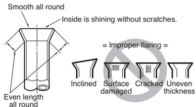
**FLARE SHAPE and FLARE NUT TIGHTENING TORQUE**
