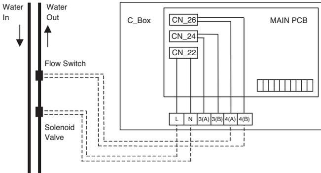
Set the DIP switch refer to Fig.1 and turn on the power when you individual control for water solenoid valve control.
