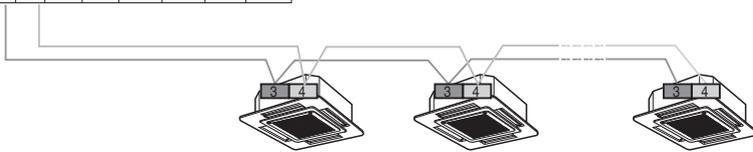
The GND terminal is a 'L' terminal for the central controller, not Ground Line
